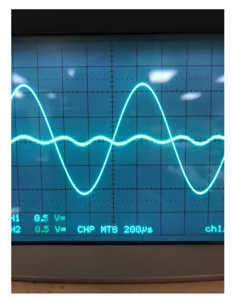
Standard Class A/B amplifier with crossover distortion
